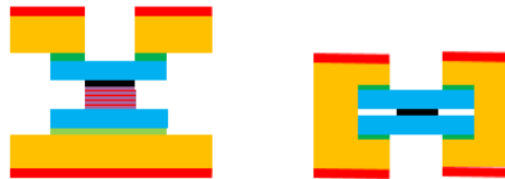
(c) Thin device VECSEL with two heatspreaders (d) DBR free SDL with two heatspreaders
